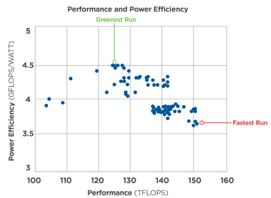
Fig. 8. Results of Linpack benchmark runs with various configurations. Each dot corresponds to a single Linpack run.
