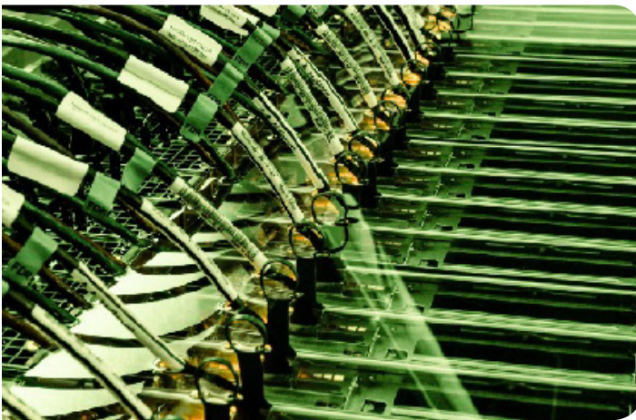
Fig. 5. The compute nodes submerged in the GRC ICERaQ system
