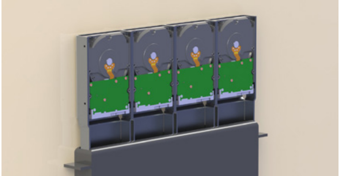
Four SuperCaddy drive elevators installed in a 1U submersion-cooled server
